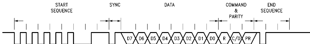
FIGURE 1-2. IBM 3270 Message Format
