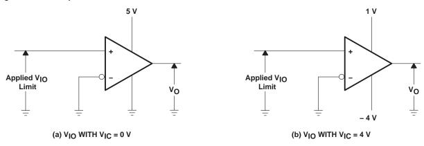
Figure 5. Method for Verifying That Input Offset Voltage Is Within Specified Limits
