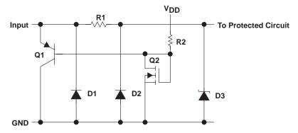
Figure 1. LinCMOS ESD-Protection Schematic
