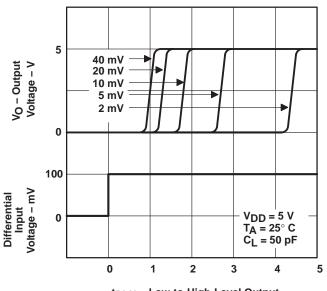
t<sub>PLH</sub> – Low-to-High-Level Output Response Time – μs
