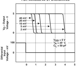
tpHL - High-to-Low-Level Output Response Time - μs
