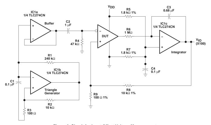
Figure 6. Circuit for Input Offset Voltage Measurement
