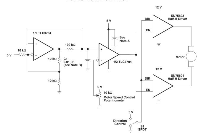
NOTES: A. The recommended minimum capacitance is 10  $\mu F$  to eliminate common ground switching noise.
