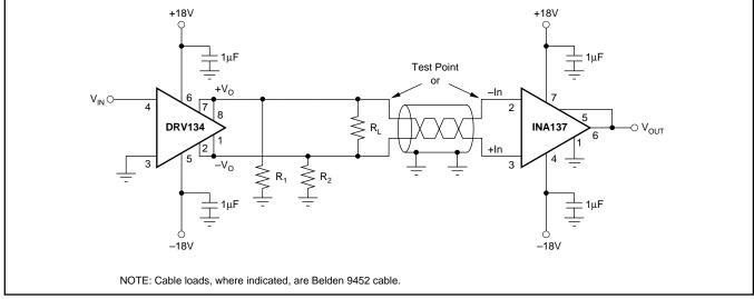
FIGURE 3. Distortion Test Circuit.
