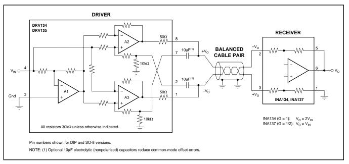
FIGURE 2. Complete Audio Driver/Receiver Circuit.
