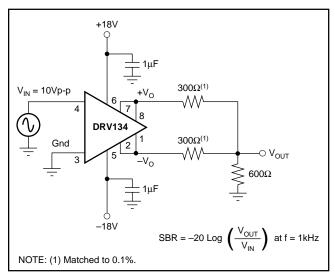
FIGURE 5. Signal Balance Ratio Test Circuit.
