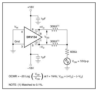
FIGURE 4. Output Common-Mode Rejection Test Circuit.
