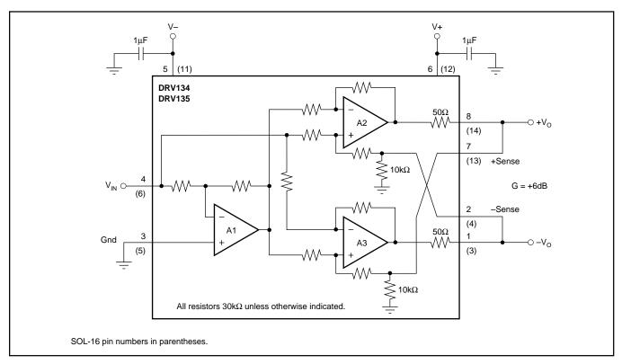
FIGURE 1. Basic Connections.
