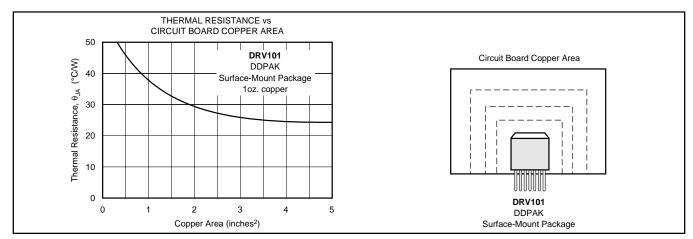
FIGURE 11. DDPAK Thermal Resistance vs Circuit Board Copper Area.
