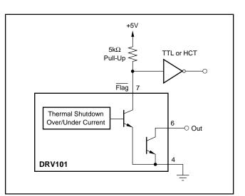
FIGURE 6. Non-Latching Fault Monitoring Circuit.
