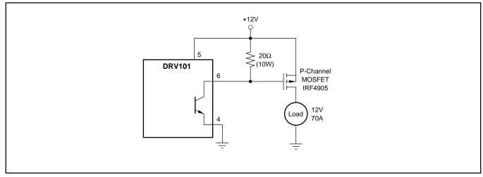
FIGURE 21. High Power, High-Side Driver.
