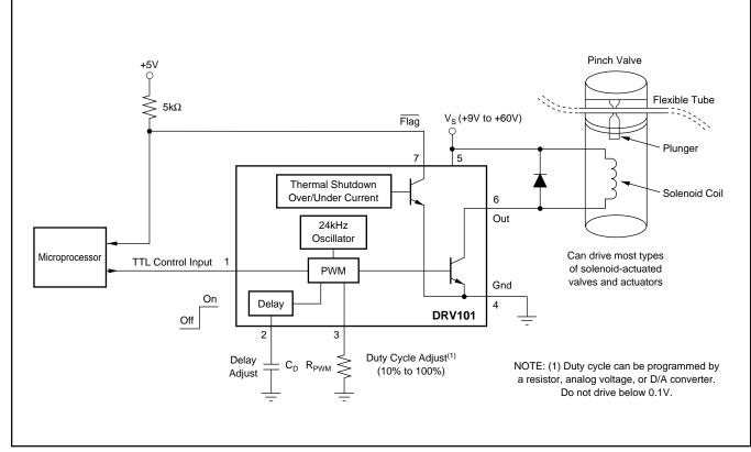
FIGURE 13. Fluid Flow Control System.
