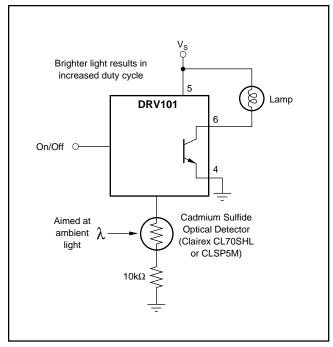
FIGURE 14. Instrument Light Dimmer Circuit.
