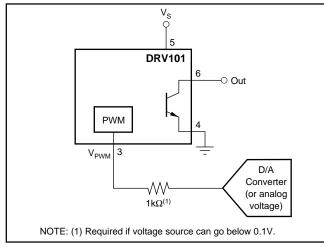
FIGURE 4. Using a Voltage to Program Duty Cycle.
