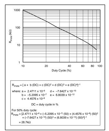
FIGURE 3. R<sub>PWM</sub> vs Duty Cycle.
