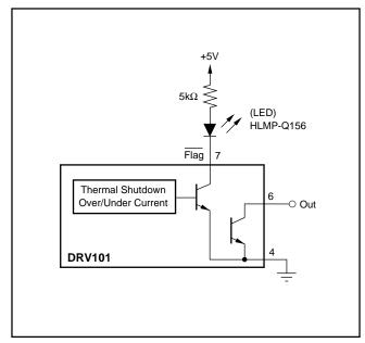
FIGURE 8. LED to Indicate Fault Condition.
