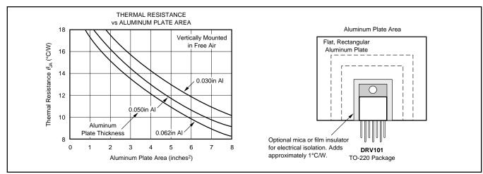
FIGURE 10. TO-220 Thermal Resistance vs Aluminum Plate Area.
