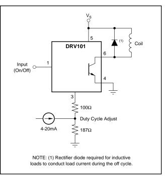
FIGURE 15. 4-20mA Input to PWM Output.
