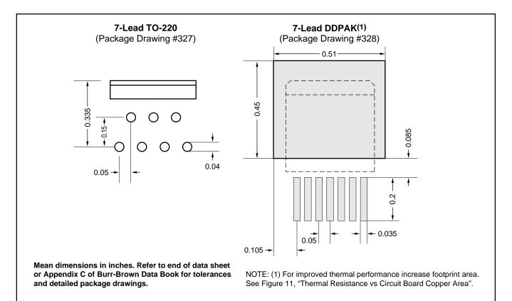
FIGURE 9. TO-220 and DDPAK Solder Footprints.
