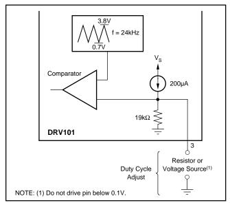
FIGURE 5. Simplified Circuit Model of the Duty Cycle Adjust Pin.
