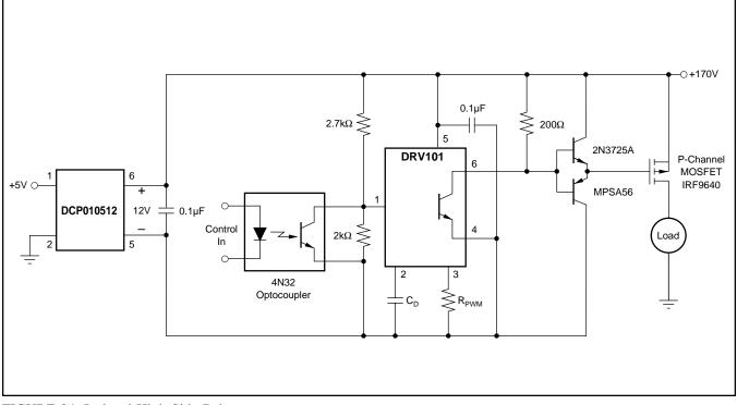
FIGURE 24. Isolated High-Side Driver.
