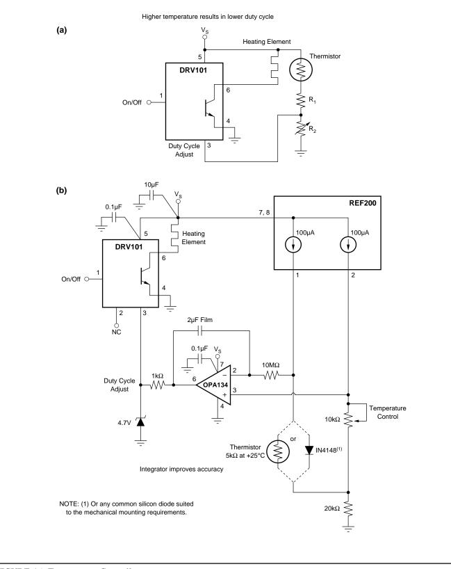
FIGURE 16. Temperature Controller.
