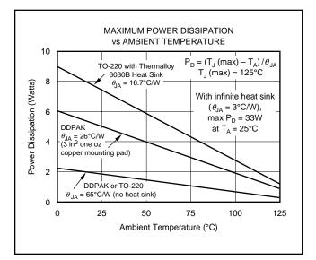
FIGURE 12. Maximum Power Dissipation vs Ambient Temperature.
