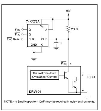
FIGURE 7. Latching Fault Monitoring Circuit.
