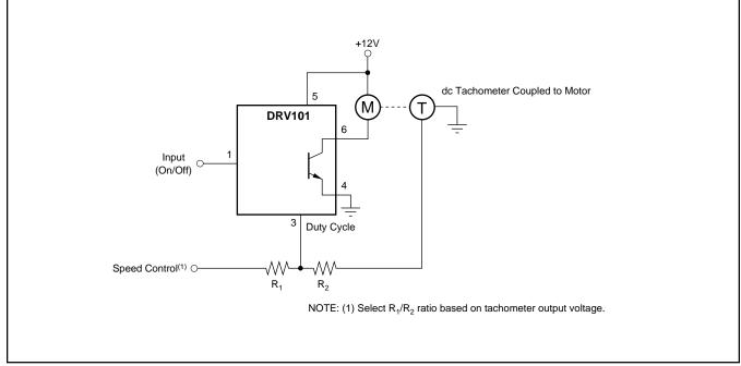
FIGURE 17. Constant Speed Motor Control.
