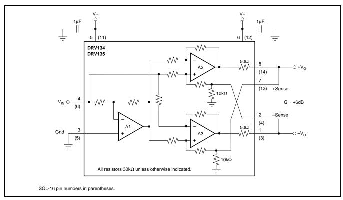
FIGURE 1. Basic Connections.
