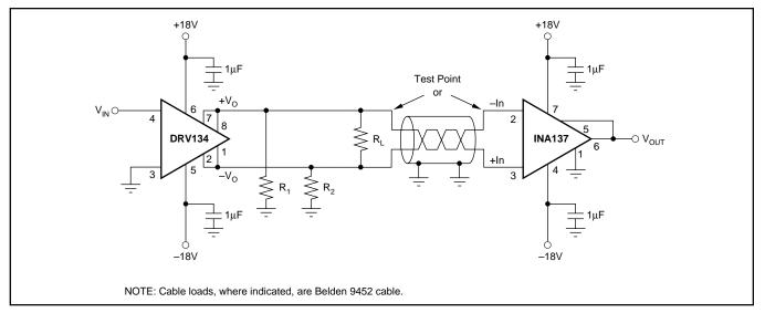
FIGURE 3. Distortion Test Circuit.
