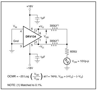
FIGURE 4. Output Common-Mode Rejection Test Circuit.
