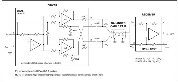
FIGURE 2. Complete Audio Driver/Receiver Circuit.
