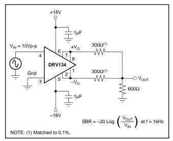
FIGURE 5. Signal Balance Ratio Test Circuit.
