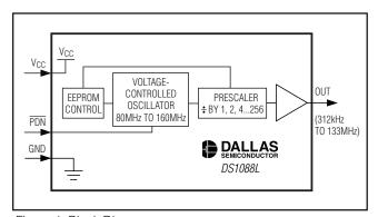
Figure 1. Block Diagram
