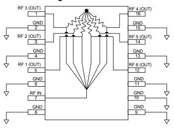
3. Pins 2, 4, 6, 8, 9, 10, 11, 13, and 15 must be DC and RF grounded.
