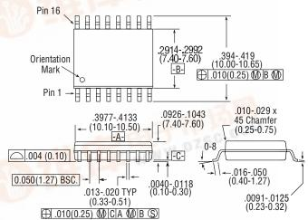
16-Lead SOP outline dimensions Wide body (.300) (All dimensions per JEDEC No. MS-013-AA, Issue C) Dimensions in ( ) are in mm.
