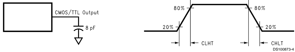
FIGURE 2. DS90CR286A/DS90CR216A (Receiver) CMOS/TTL Output Load and Transition Times
