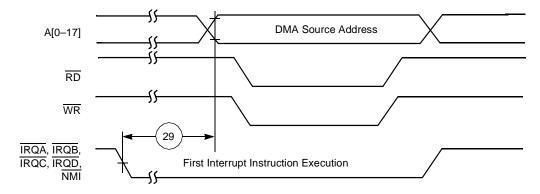
Figure 2-11. External Memory Access (DMA Source) Timing
