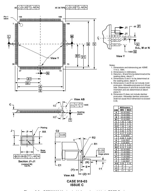
Figure 3-3. DSP56309 Mechanical Information, 144-pin TQFP Package
