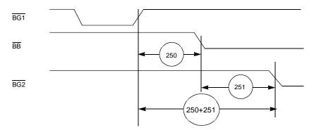
Figure 2-26. Asynchronous Bus Arbitration Timing
