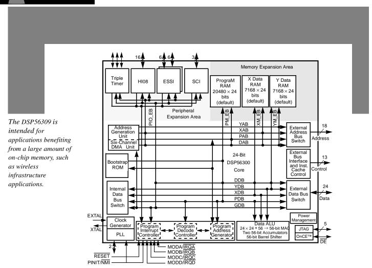
Figure 1. DSP56309 Block Diagram
