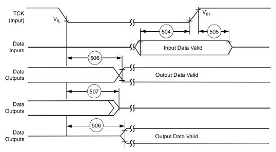
Figure 2-45. Boundary Scan (JTAG) Timing Diagram
