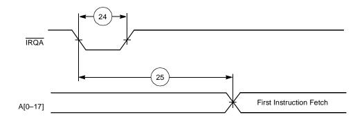
Figure 2-9. Recovery from Stop State Using IRQA
