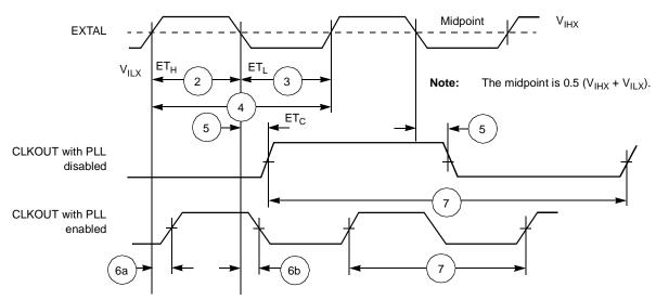
Figure 2-2. External Clock Timing
