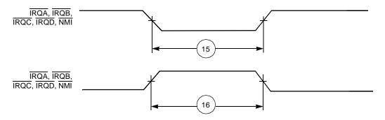
Figure 2-6. External Interrupt Timing (Negative Edge-Triggered)
