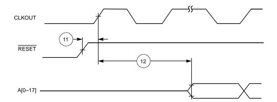
Figure 2-4. Synchronous Reset Timing
