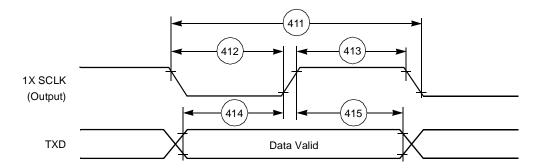
Figure 2-37. SCI Asynchronous Mode Timing
