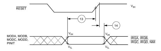
Figure 2-8. Operating Mode Select Timing
