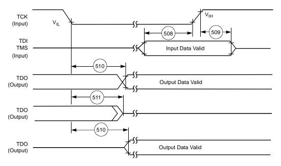
Figure 2-46. Test Access Port Timing Diagram
