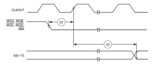
Figure 2-7. Synchronous Interrupt from Wait State Timing
