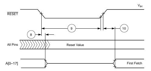
Figure 2-3. Reset Timing
