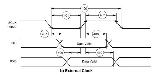
Figure 2-36. SCI Synchronous Mode Timing
