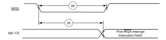
Figure 2-10. Recovery from Stop State Using IRQA Interrupt Service
