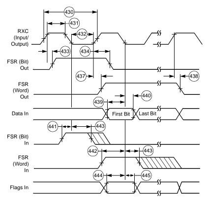
Figure 2-39. ESSI Receiver Timing
