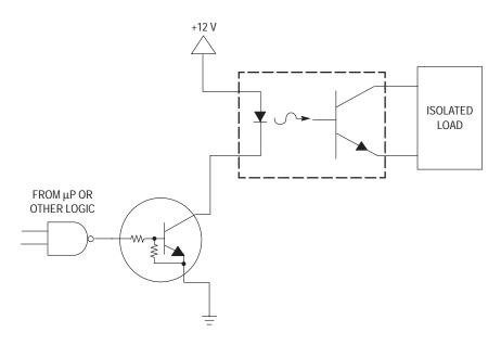
Figure 23. Level Shifter: Connects 12 or 24 Volt Circuits to Logic
