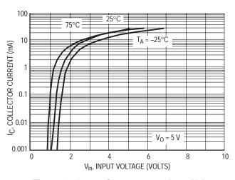
Figure 16. Output Current versus Input Voltage
