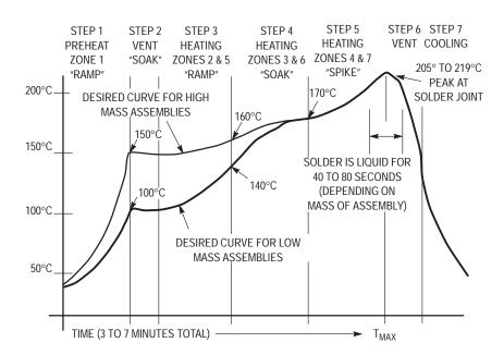
Figure 26. Typical Solder Heating Profile
