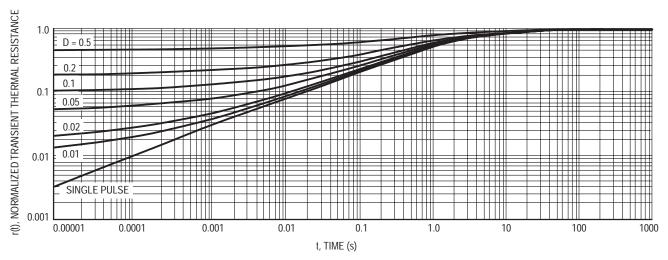
Figure 2. Normalized Thermal Response
