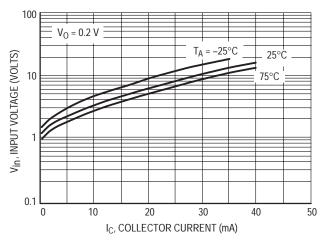
Figure 17. Input Voltage versus Output Current
