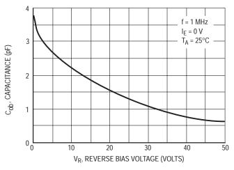
Figure 5. Output Capacitance
