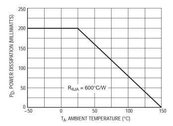
Figure 1. Derating Curve
