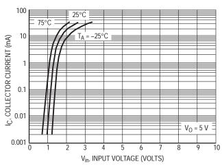
Figure 6. Output Current versus Input Voltage
