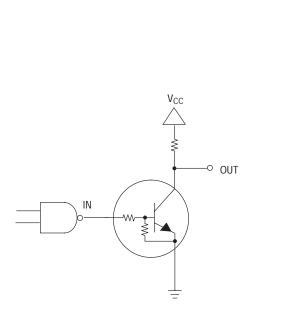
Figure 24. Open Collector Inverter: Inverts the Input Signal
