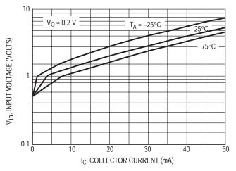
Figure 22. Input Voltage versus Output Current
