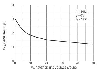
Figure 10. Output Capacitance
