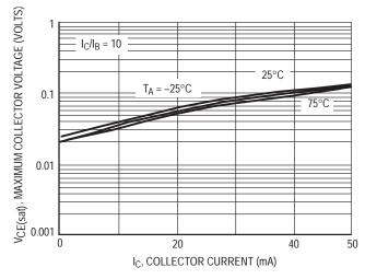
Figure 8. V<sub>CE(sat)</sub> versus I<sub>C</sub>
