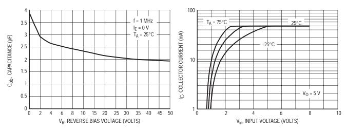
Figure 20. Output Capacitance
