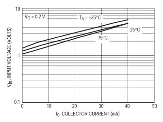
Figure 7. Input Voltage versus Output Current
