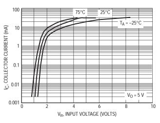
Figure 11. Output Current versus Input Voltage
