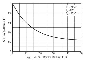
Figure 15. Output Capacitance
