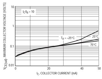
Figure 13.  $V_{CE(sat)}$  versus  $I_C$
