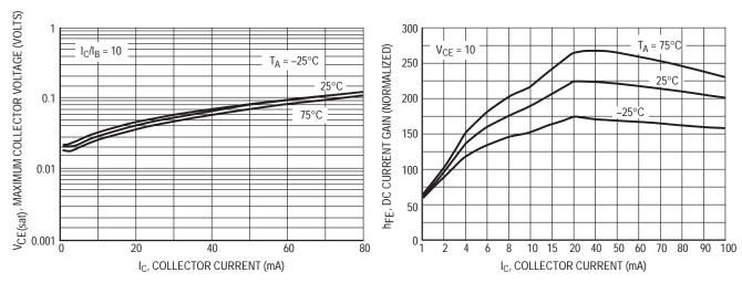
Figure 18. V<sub>CE(sat)</sub> versus I<sub>C</sub>
