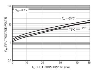
Figure 12. Input Voltage versus Output Current
