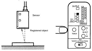
Position the registered object at the detection point and press the TEACH button.
