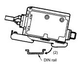
Press the E3MC in the direction indicated by arrow (3) and slide part A in the direction indicated by arrow (4) as shown in the following illustration until the E39-L115 correctly engages with the DIN rail.
