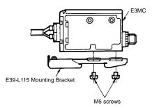
2. When mounting the E3MC with the E39-L115, loosen the M3 screw of the E39-L115 and slide part A in the direction indicated by arrow (1) as shown in the following illustration.
