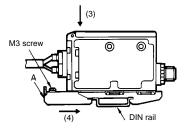
Tighten the M3 screw of the E39-L115 to secure the E39-L115.
