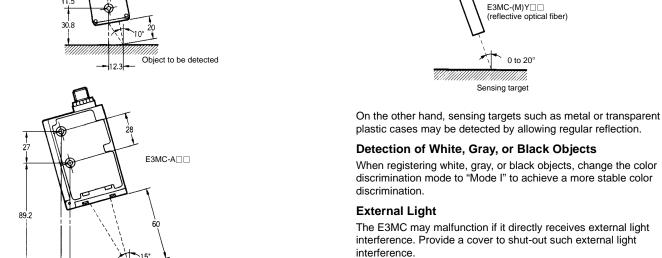
Note: To avoid malfunction, provide a cover to shut out direct external light interference to the E3MC.
