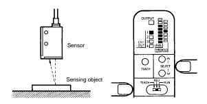
Press the SELECT button in ADJ mode with or without the object to be detected positioned at the detection point. The channel selected in the TEACH mode or RUN mode will become the channel for the ADJ mode.
