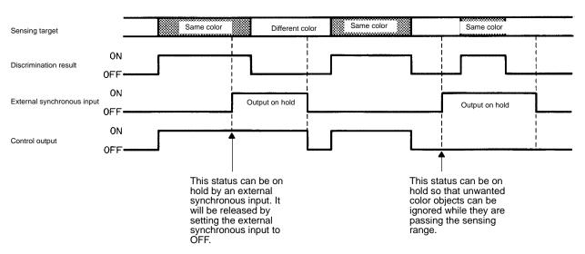
Note: External Synchronous Input: Latches sensor output in existing state when ESI is on. For example, if sensor output is on when ESI is on, the output(s) will remain on until ESI is turned off, regardless of target presence or absence.
