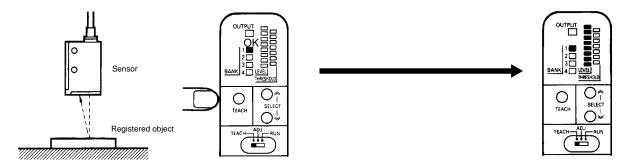
Position the registered object at the detection point and press the TEACH button.
