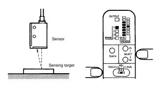
Press the SELECT button in ADJ mode with or without the object to be detected positioned at the detection point.
