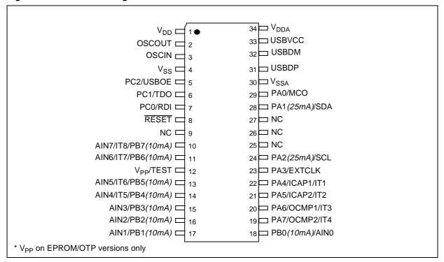
Figure 3. 32-Pin SDIP Package Pinout
