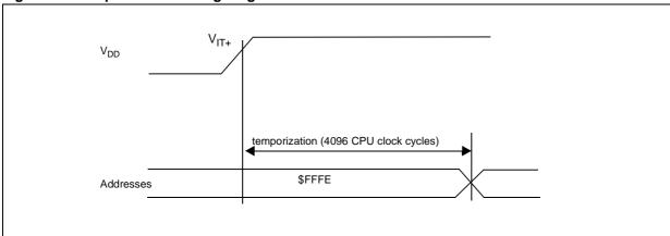
Figure 14. Reset Timing Diagram
