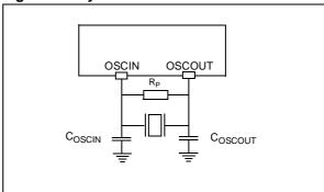
Figure 10. Clock block diagram
