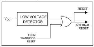
Figure 12. Low Voltage Reset Signal Output
