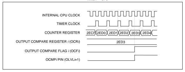
Figure 31. Output Compare Timing Diagram, f<sub>TIMER</sub> =f<sub>CPU</sub>/4
