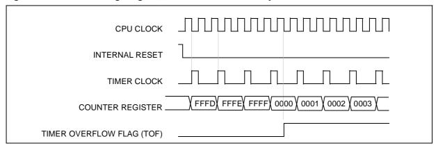
Figure 25. Counter Timing Diagram, internal clock divided by 4
