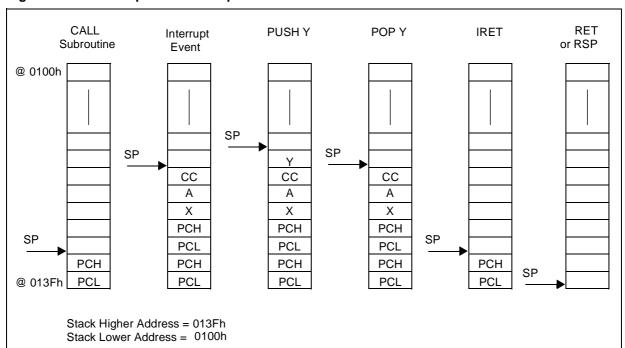
Figure 7. Stack Manipulation Example
