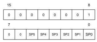
The Stack Pointer is a 16-bit register which is always pointing to the next free location in the stack. It is then decremented after data has been pushed onto the stack and incremented before data is popped from the stack (see Figure 7).
