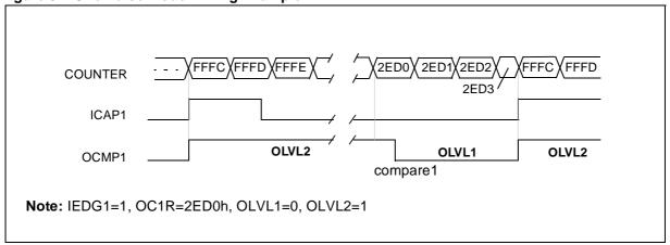
Figure 33. Pulse Width Modulation Mode Timing Example
