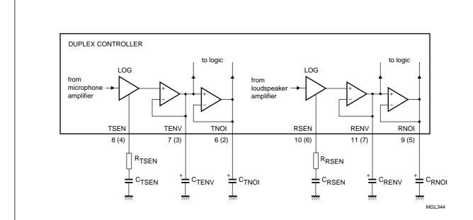
Pin numbers in parenthesis apply to the TEA1098H. Pin numbers not in parenthesis apply to the TEA1098TV.
