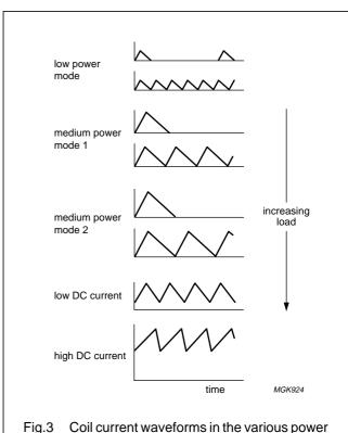
Fig.3 Coil current waveforms in the various power modes.
