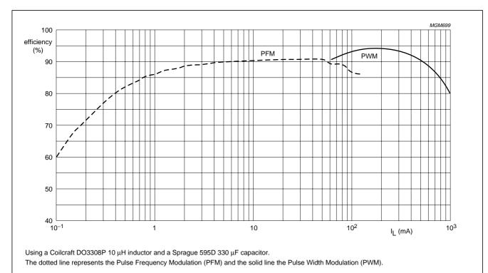
Fig.6 Efficiency as a function of load current  $I_L$  (2.4 to 3.3 V).
