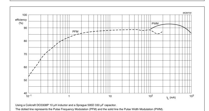
Fig.7 Efficiency as a function of load current  $\rm I_L$  (3.6 to 5.5 V).
