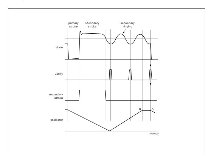
A: Start of new cycle at lowest drain voltage.
