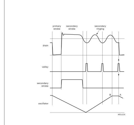
A: Start of new cycle at lowest drain voltage.
