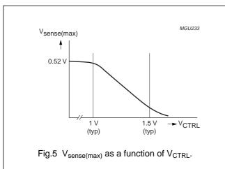
The maximum fixed frequency of the oscillator is set by an internal current source and capacitor. The maximum frequency is reduced once the control voltage enters the VCO control window. Then, the maximum frequency changes linearly with the control voltage until the minimum frequency is reached (see Figs 5 and 6).
