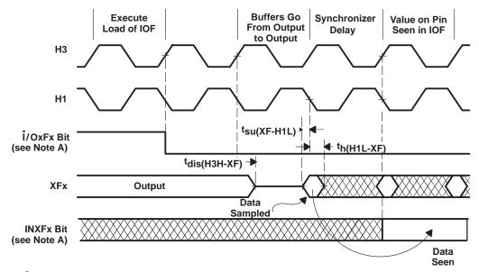
NOTE A: 1/OxFx represents either bit 1 or bit 5 of the IOF register, and INXFx represents either bit 3 or bit 7 of the IOF register.
