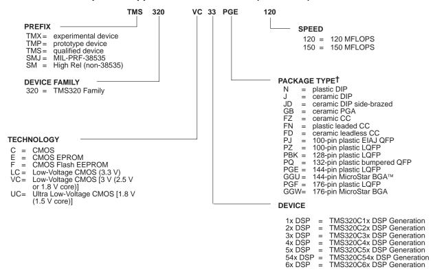
† DIP = Dual-In-Line Package PGA = Pin Grid Array CC = Chip Carrier QFP = Quad Flat Package LQFP = Low-Profile Quad Flat Package BGA = Ball Grid Array
