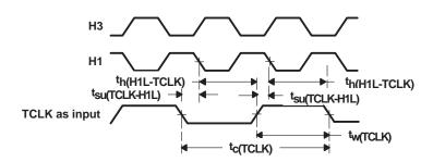
Figure 37. Timer Pin Timing, Input
