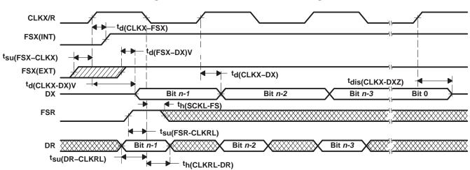
Figure 31. Fixed Data-Rate Mode Timing
