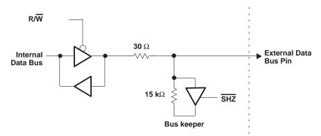
Figure 9. Bus Keeper Circuit
