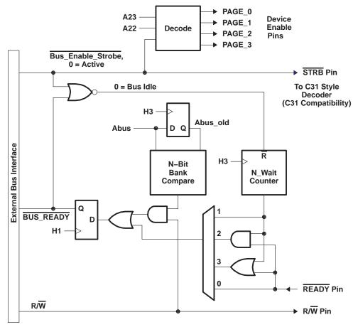
Figure 8. Internal Ready Logic, Simplified Diagram
