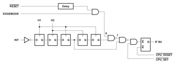
Figure 7. EDGEMODE and Interrupt Flag Circuit
