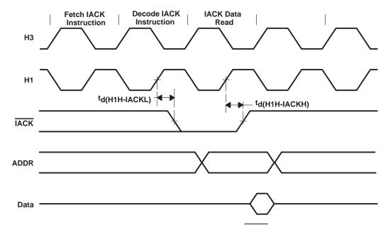
Figure 30. Interrupt Acknowledge (IACK) Timing
