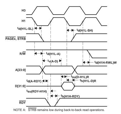
Figure 20. Timing for Memory ( $\overline{STRB} = 0$  and  $\overline{PAGEx} = 0$ ) Read
