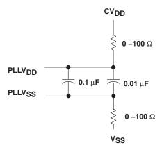
Figure 6. PLL Isolation Circuit Diagram
