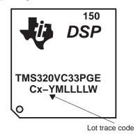
Figure 13. PGE Package (Top View)
