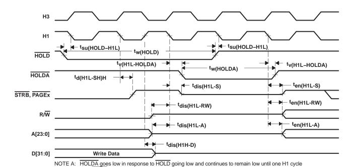
Figure 33. Timing for HOLD/HOLDA (After Write)
