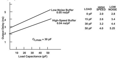
Figure 19. Output Load Characteristics, Buffer Only
