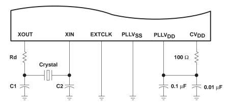
Figure 5. Self-Oscillation Mode
