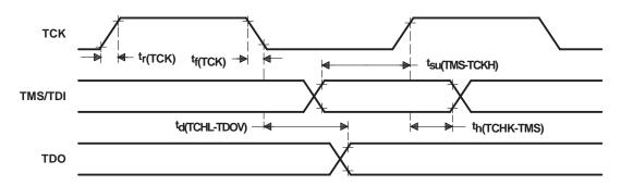
Figure 40. IEEE-1149.1 Test Access Port Timings
