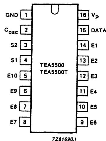
Fig. 2 Pinning diagram.
