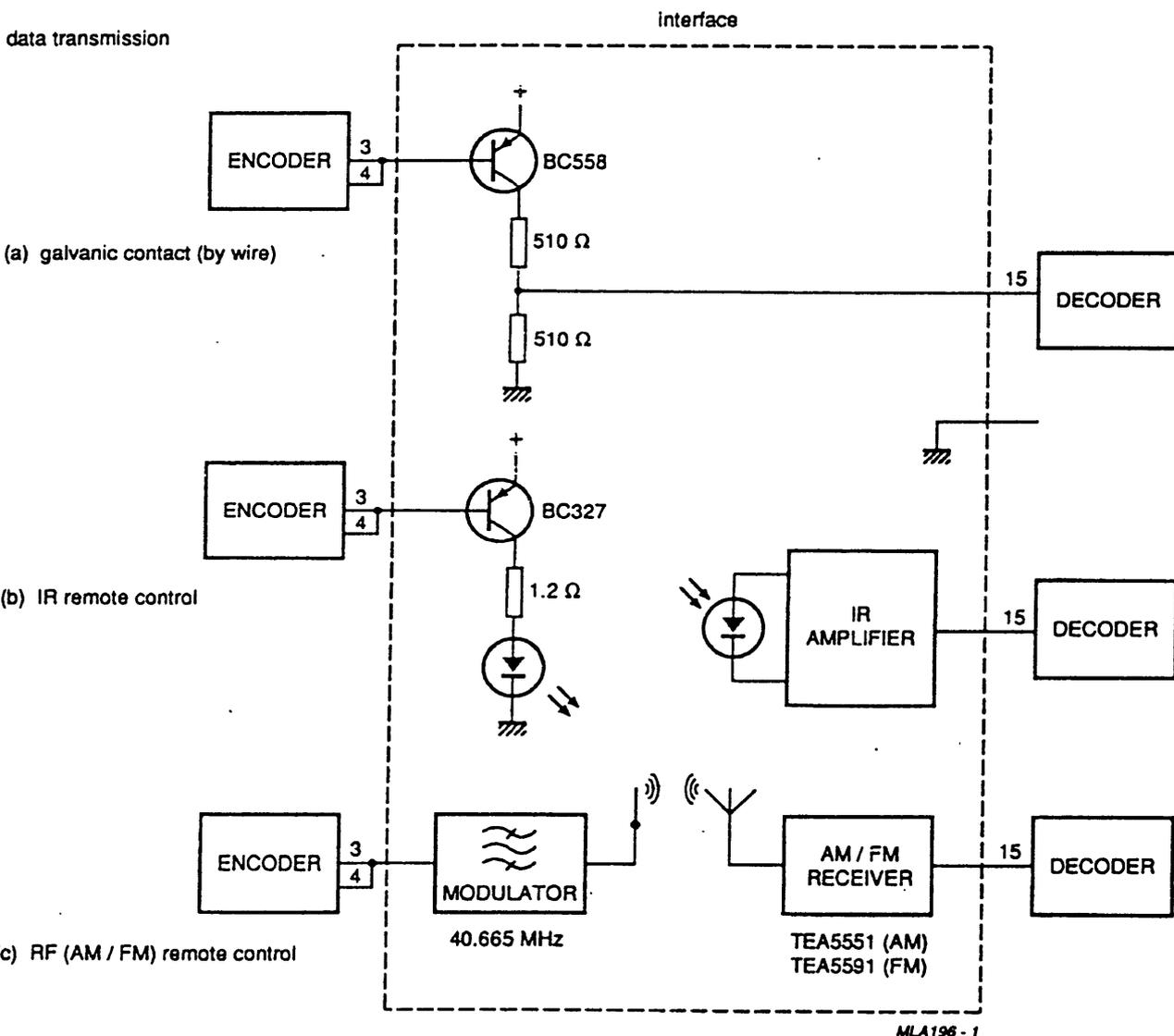
Fig. 7 Application diagram; types of data transmission possible by using different interfaces.
