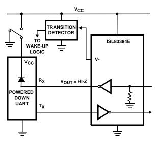
FIGURE 3. DISABLED RECEIVERS PREVENT POWER DRAIN
