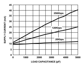
FIGURE 11. SUPPLY CURRENT vs LOAD CAPACITANCE WHEN TRANSMITTING DATA
