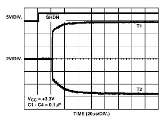
FIGURE 5. TRANSMITTER OUTPUTS WHEN EXITING POWERDOWN
