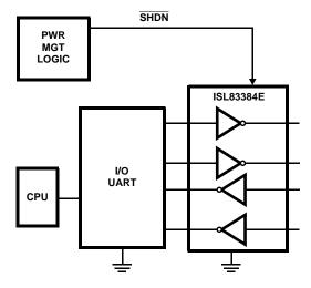
FIGURE 4. CONNECTIONS FOR MANUAL POWERDOWN
