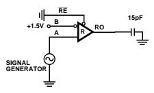
FIGURE 4A. TEST CIRCUIT
