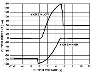
FIGURE 8. DRIVER OUTPUT CURRENT vs SHORT CIRCUIT **VOLTAGE**
