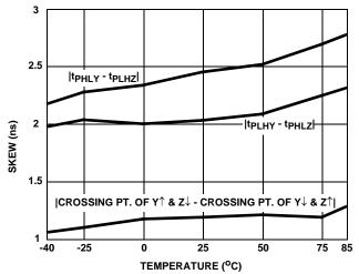
FIGURE 13. DRIVER SKEW vs TEMPERATURE (ISL8485E)
