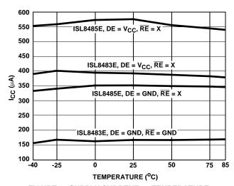
FIGURE 9. SUPPLY CURRENT vs TEMPERATURE
