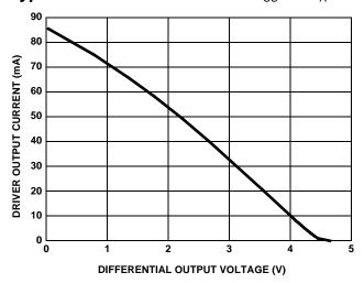
FIGURE 6. DRIVER OUTPUT CURRENT vs DIFFERENTIAL **OUTPUT VOLTAGE**
