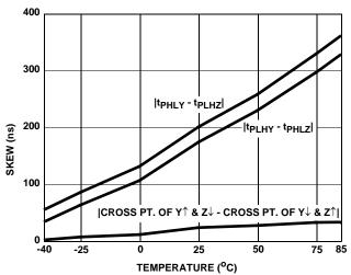
FIGURE 11. DRIVER SKEW vs TEMPERATURE (ISL8483E)
