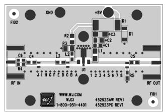
Circuit Board Material: .014" Getek, 4 - layer, 1 oz copper, Microstrip line details: width = .026", spacing = .026" The silk screen markers 'A', 'B', 'C', etc. and '1', '2', '3', etc. are used as placemarkers for the input and output tuning shunt capacitors. The markers and vias are spaced in .050" increments.
