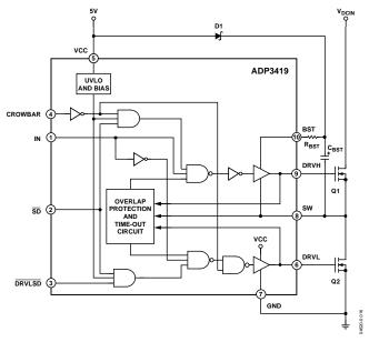
Figure 17. Detailed Block Diagram of the ADP3419
