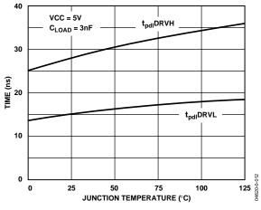
Figure 13. DRVH and DRVL t<sub>pdl</sub> vs. Temperature
