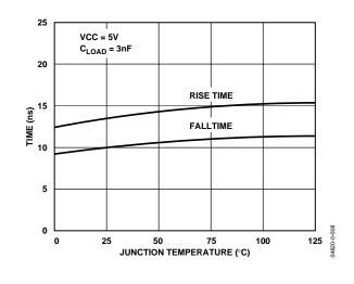
Figure 9. DRVL Rise and Fall Times vs. Temperature
