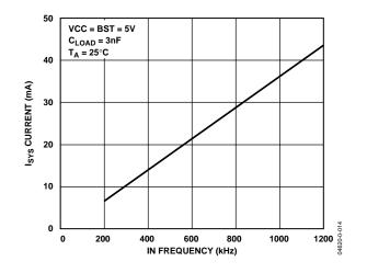
Figure 15. Supply Current vs. Frequency
