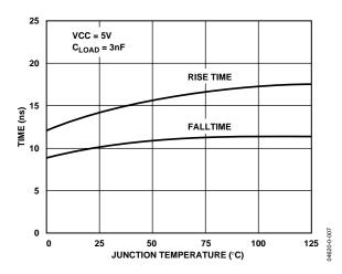
Figure 8. DRVH Rise and Fall Times vs. Temperature
