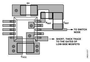
Figure 18. External Component Placement Example
