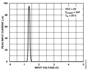
Figure 14. IN Pin Input Current vs. Input Voltage
