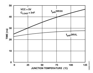
Figure 12. DRVH and DRVL t<sub>pdh</sub> vs. Temperature
