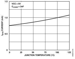
Figure 16. Supply Current vs. Temperature
