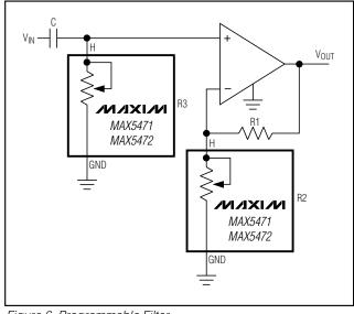
Figure 6. Programmable Filter
