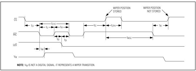
Figure 1. Digital Interface and Timing Diagram
