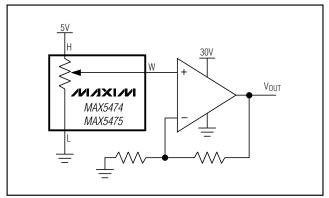
Figure 4. Positive LCD Bias Control Using a Voltage-Divider
