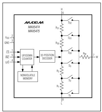
Figure 3. MAX5474/MAX5475 Functional Diagram
