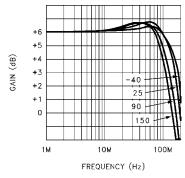
FIGURE 3. FREQUENCY RESPONSE vs TEMPERATURE
