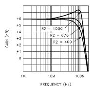
FIGURE 2. FREQUENCY RESPONSE vs RESISTOR R2 (GAIN = 2)
