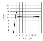
FIGURE 1. IS vs SUPPLY VOLTAGE
