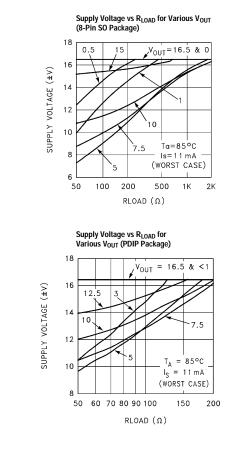
The curves do not include heat removal or forcing air, or the simple fact that the package will probably be attached to a circuit board, which can also provide some form of heat removal. Larger temperature and voltage ranges are possible with heat removal and forcing air past the part.
