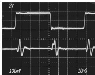
Switching Glitch, 0V to 0V with 2ns AB edges
