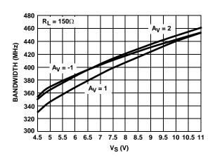
FIGURE 11. BANDWIDTH vs SUPPLY VOLTAGE
