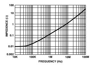
FIGURE 8. OUTPUT IMPEDENCE vs FREQUENCY
