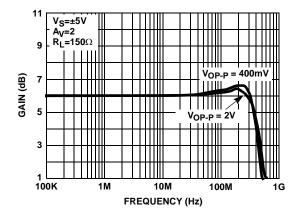
FIGURE 3. FREQUENCY RESPONSE vs OUTPUT VOLTAGE
