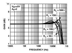
FIGURE 4. FREQUENCY RESPONSE vs RL
