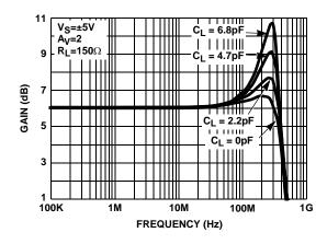
FIGURE 5. FREQUENCY RESPONSE FOR VARIOUS CL
