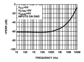
FIGURE 7. PSRR vs FREQUENCY
