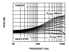
FIGURE 8. GAIN AS THE FUNCTION OF  $V_{\mbox{CTRL}}$
