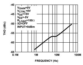
FIGURE 2. TOTAL HARMONIC DISTORTION
