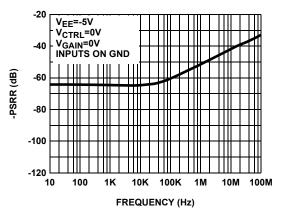
FIGURE 6. PSRR vs FREQUENCY
