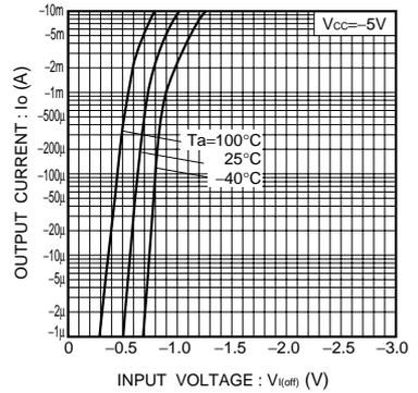
Fig.6 Output current vs. input voltage (OFF characteristics)
