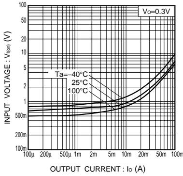
Fig.1 Input voltage vs. output current (ON characteristics)
