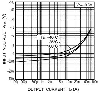
Fig.5 Input voltage vs. output current (ON characteristics)
