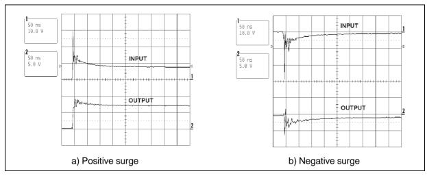
Please note that the EMIF01-10005W5 is not only acting for positive ESD surges but also for negative ones. For these kind of disturbances it clamps close to ground voltage as shown in Fig. A5b.
