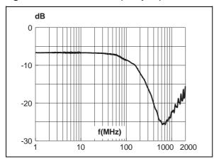
Figure A1 gives these parameters, in particular the signal rejection at the GSM frequency is about -24dB at 900MHz,
