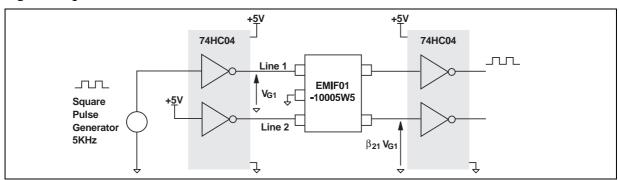
Figure A8 shows the measurement circuit used to quantify the crosstalk effect in a classical digital application.
