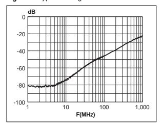
Figure A10 gives the measurement circuit for the analog application. In figure A11, the curve shows the effect of cell I/O1 on cell I/O2. In usual frequency range of analog signals (up to 100MHz) the effect on disturbed line is less than -43 dB.
