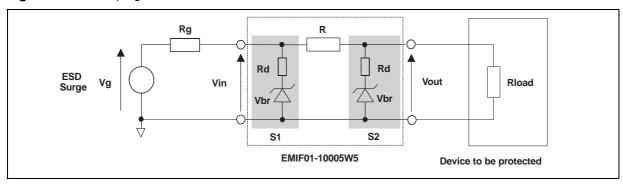
To have a good approximation of the remaining voltages at both Vin and Vout stages, we provide the typical dynamical resistance value Rd. By taking into account these following hypothesis: R>>Rd, RG>>Rd and Rload>>Rd, it gives these formulas:
