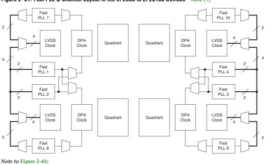
Figure 2–61. Fast PLL & Channel Layout in the EP2S60 to EP2S180 Devices Note (1)
