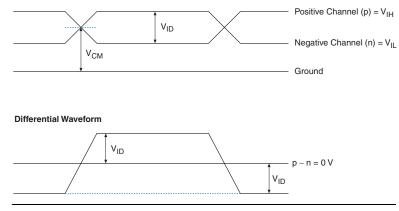
Figure 5–2. Transmitter Output Waveforms for Differential I/O Standards
