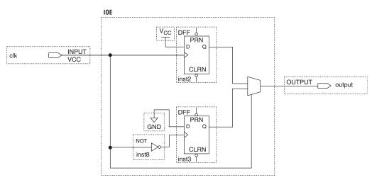
Figure 5–9. DCD Measurement Technique for DDIO (Double-Data Rate) Outputs
