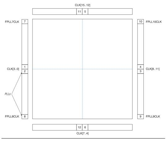
Figures 2–41 and 2–42 shows the global and regional clocking from the fast PLL outputs and the side clock pins. The connections to the global and regional clocks from the fast PLL outputs, internal drivers, and the CLK pins on the left and right sides of the device are shown in table format in Tables 2–11 and 2–12, respectively.
