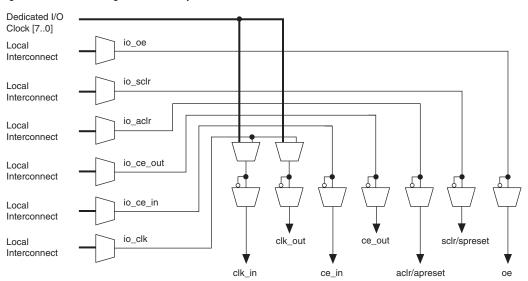
Figure 2–50. Control Signal Selection per IOE
