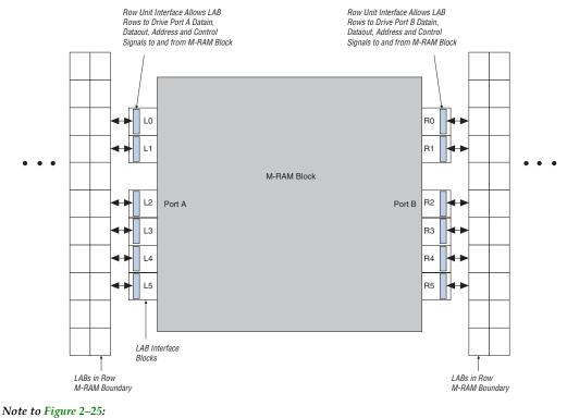
Figure 2–25. M-RAM Block LAB Row Interface Note (1)
