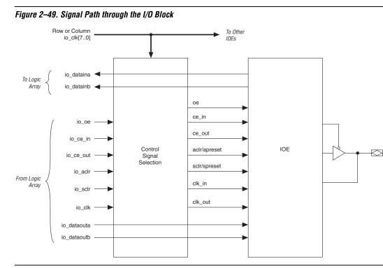
Each IOE contains its own control signal selection for the following control signals: oe, ce\_in, ce\_out, aclr/apreset, sclr/spreset, clk\_in, and clk\_out. Figure 2–50 illustrates the control signal selection.
