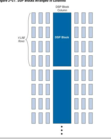
Figure 2–27. DSP Blocks Arranged in Columns
