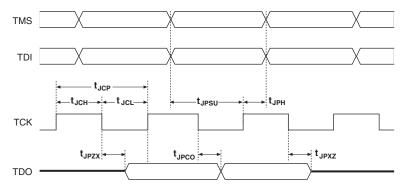
Table 5–102 shows the JTAG timing parameters and values for Stratix II devices.
