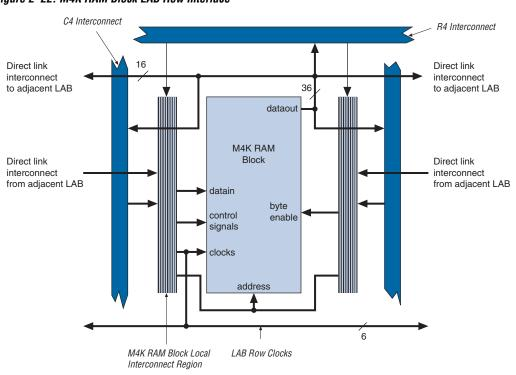
Figure 2–22. M4K RAM Block LAB Row Interface
