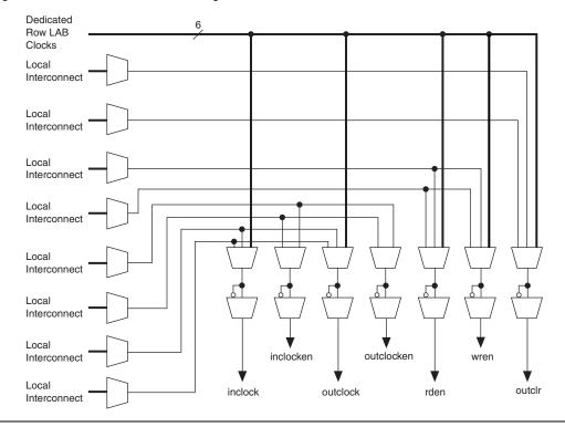
Figure 2–19. M512 RAM Block Control Signals
