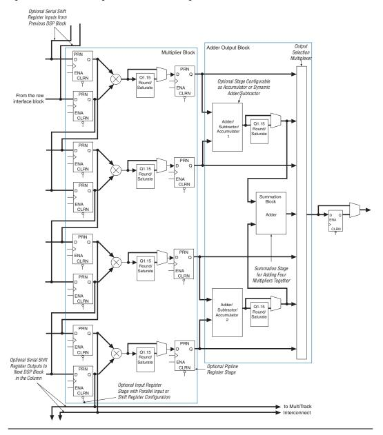
Figure 2–28. DSP Block Diagram for 18 × 18-Bit Configuration
