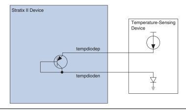
Figure 3–1. External Temperature-Sensing Diode
