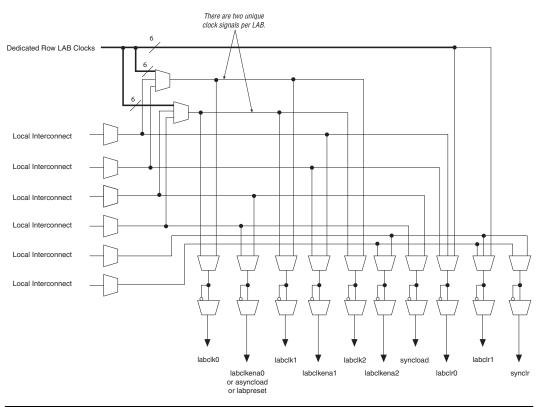
Figure 2–4. LAB-Wide Control Signals
