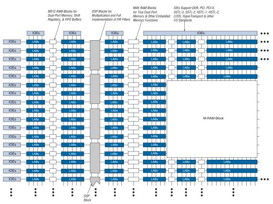
Figure 2–1. Stratix II Block Diagram
