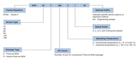
Figure 6–1. Stratix II Device Packaging Ordering Information
