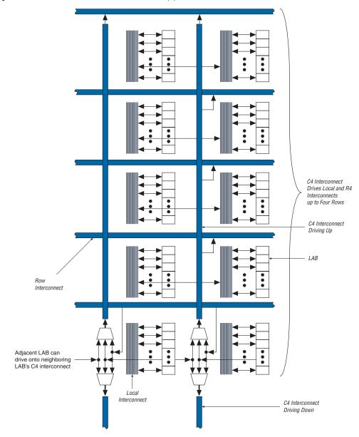
Figure 2–18. C4 Interconnect Connections Note (1)
