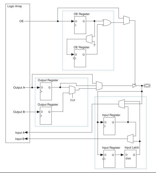
The IOEs are located in I/O blocks around the periphery of the Stratix II device. There are up to four IOEs per row I/O block and four IOEs per column I/O block. The row I/O blocks drive row, column, or direct link interconnects. The column I/O blocks drive column interconnects. Figure 2–47 shows how a row I/O block connects to the logic array. Figure 2–48 shows how a column I/O block connects to the logic array.
