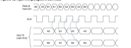
Figure 2–53. Input Timing Diagram in DDR Mode
