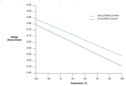
Figure 3–2. Temperature vs. Temperature-Sensing Diode Voltage
