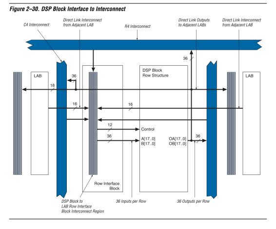
A bus of 44 control signals feeds the entire DSP block. These signals include clocks, asynchronous clears, clock enables, signed/unsigned control signals, addition and subtraction control signals, rounding and saturation control signals, and accumulator synchronous loads. The clock
