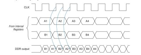
The Stratix II IOE operates in bidirectional DDR mode by combining the DDR input and DDR output configurations. The negative-edge-clocked OE register holds the OE signal inactive until the falling edge of the clock. This is done to meet DDR SDRAM timing requirements.
