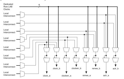
Figure 2–21. M4K RAM Block Control Signals
