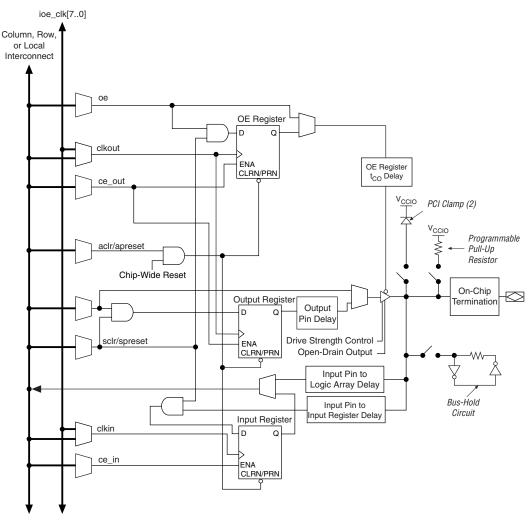
Figure 2–51. Stratix II IOE in Bidirectional I/O Configuration Note (1)
