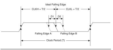
DCD expressed in absolution derivation, for example, D1 or D2 in Figure 5–7, is clock-period independent. DCD can also be expressed as a percentage, and the percentage number is clock-period dependent. DCD as a percentage is defined as
