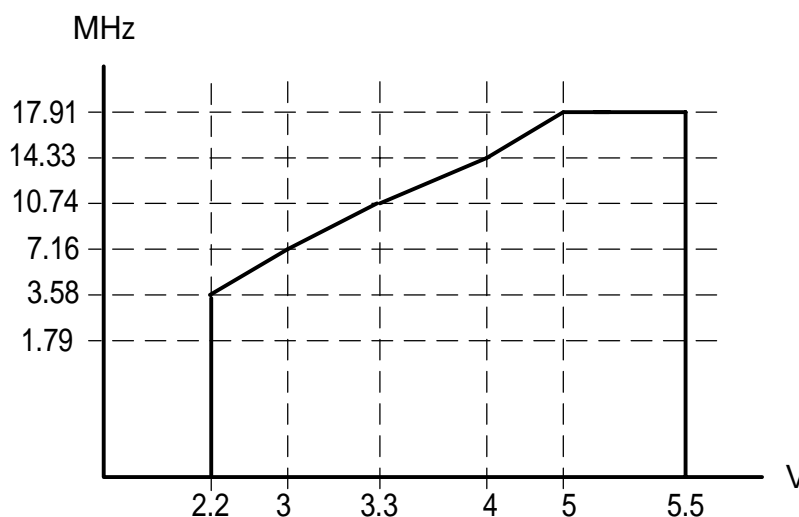
Fig. 16 Operation Voltage XY Axis
