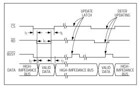
Figure 9. MX7576 Asynchronous Conversion Mode Timing Diagram
