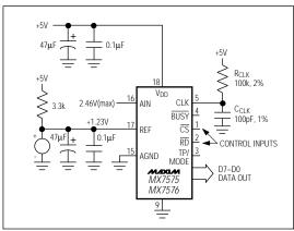
Figure 16a. Unipolar Configuration
