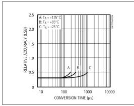
Figure 14. MX7575 Accuracy vs. Conversion Time
