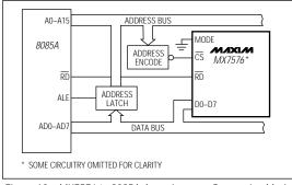
Figure 10. MX7576 to 8085A Asynchronous Conversion Mode Interface
