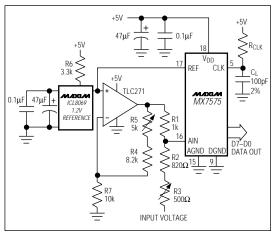
Figure 18a. MX7575 Bipolar Configuration
