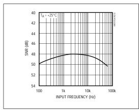
Figure 13. MX7575 SNR vs. Input Frequency
