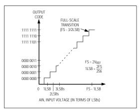
Figure 16b. Nominal Transfer Characteristic for Unipolar Operation
