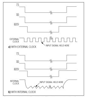
Figure 12. MX7575 Track/Hold (Slow-Memory Interface) Timing Diagrams
