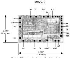
\*The two AGND pads must both be used (bonded together).
