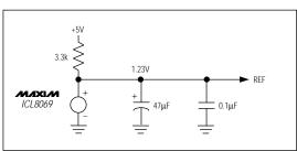
Figure 15. External Reference Circuit
