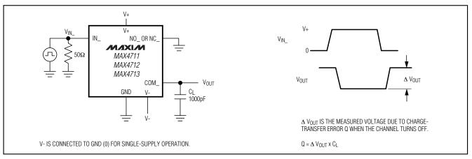
Figure 4. Charge Injection
