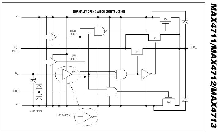
Figure 1. Block Diagram
