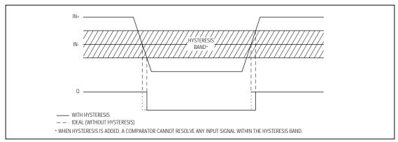
Figure 2. Effect of Hysteresis on Input Resolution
