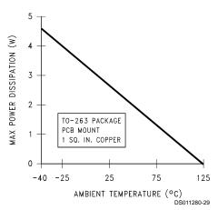
FIGURE 4. Maximum Power Dissipation vs T<sub>AMB</sub> for the TO-263 Package
