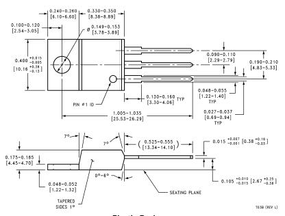
Plastic Package Order Number LM2937ET-5.0, LM2937ET-8.0, LM2937ET-10, LM2937ET-12, or LM2937ET-15 NS Package Number T03B
