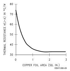
FIGURE 3.  $\theta_{\text{(J-A)}}$  vs Copper (1 ounce) Area for the TO-263 Package
