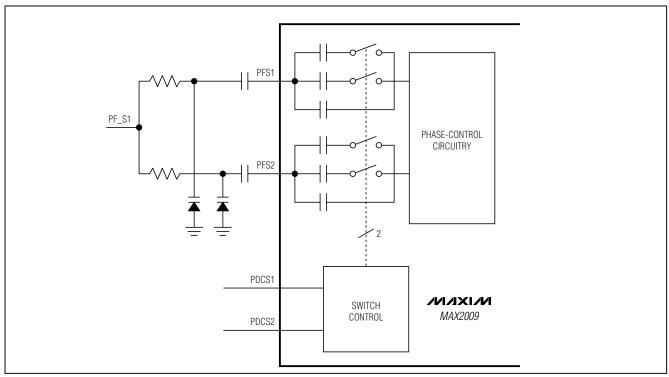
Figure 2. Simplified Phase Slope Internal Circuitry
