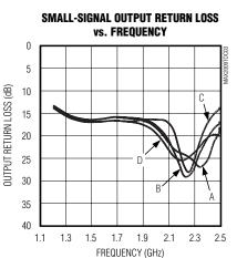
A = V<sub>PDCS1</sub> = V<sub>PDCS2</sub> = V<sub>PF\_S1</sub> = 0V B = V<sub>PDCS1</sub> = V<sub>PDCS2</sub> = 0V, V<sub>PF\_S1</sub> = 5V C = V<sub>PDCS1</sub> = V<sub>PDCS2</sub> = 5V, V<sub>PF\_S1</sub> = 0V  $D = V_{PDCS1} = V_{PDCS2} = V_{PF\_S1} = 5V$
