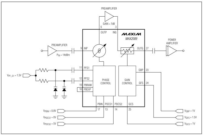
Figure 5. MAX2009 Phase and Gain Optimization Circuit
