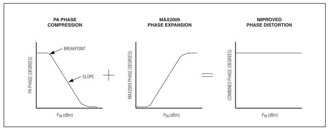
Figure 1. PA Phase Compression Canceled by MAX2009 Phase Expansion
