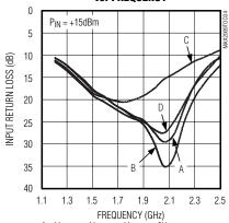
A = V<sub>PDCS1</sub> = V<sub>PDCS2</sub> = V<sub>PF\_S1</sub> = 0V B = V<sub>PDCS1</sub> = V<sub>PDCS2</sub> = 0V, V<sub>PF\_S1</sub> = 5V C = V<sub>PDCS1</sub> = V<sub>PDCS2</sub> = 5V, V<sub>PF\_S1</sub> = 0V D = V<sub>PDCS1</sub> = V<sub>PDCS2</sub> = V<sub>PF\_S1</sub> = 5V
