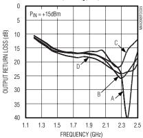
A = V<sub>PDCS1</sub> = V<sub>PDCS2</sub> = V<sub>PF\_S1</sub> = 0V B = V<sub>PDCS1</sub> = V<sub>PDCS2</sub> = 0V, V<sub>PF\_S1</sub> = 5V C = V<sub>PDCS1</sub> = V<sub>PDCS2</sub> = 5V, V<sub>PF\_S1</sub> = 0V D = V<sub>PDCS1</sub> = V<sub>PDCS2</sub> = V<sub>PF\_S1</sub> = 5V
