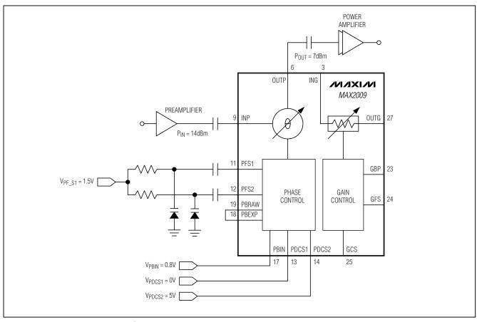
Figure 4. AM-PM Response Tuning Circuit
