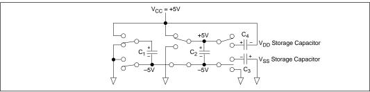
Figure 18. Charge Pump — Phase 3
