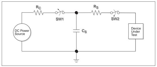
Figure 20. ESD Test Circuit for Human Body Model
