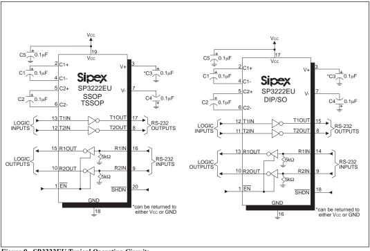
Figure 9. SP3222EU Typical Operating Circuits
