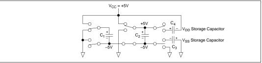
Figure 15. Charge Pump — Phase 1
