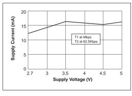
Figure 4. Supply Current vs Supply Voltage for the SP3222EU and the SP3232EU
