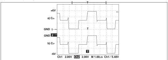
Figure 17. Charge Pump Waveforms
