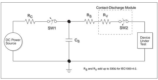
Figure 21. ESD Test Circuit for IEC1000-4-2
