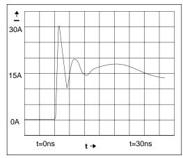
Figure 22. ESD Test Waveform for IEC1000-4-2
