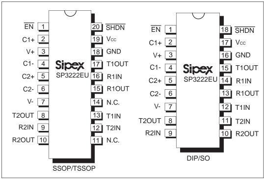
Figure 7. Pinout Configurations for the SP3222EU
