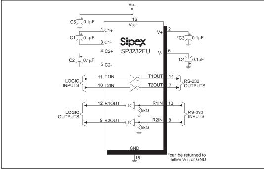
Figure 10. SP3232EU Typical Operating Circuit
