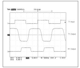
Figure 13. Driver Loopback Test One Driver 1Mbps
