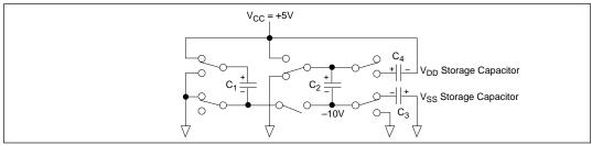
Figure 16. Charge Pump — Phase 2
