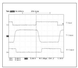
Figure 12. Driver Loopback Test All Drivers at 250kbps
