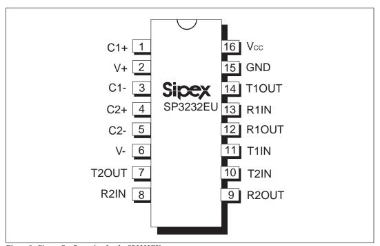
Figure 8. Pinout Configuration for the SP3232EU
