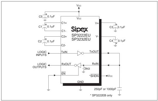
Figure 11. SP3222EU/3232EU Driver Loopback Test Circuit
