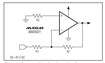
Figure 1b. Reducing Offset Error Due to Bias Current (Inverting)
