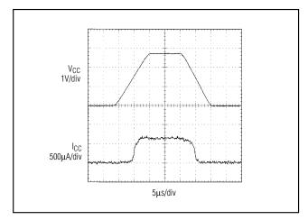
Figure 10. Power-Up Supply Current
