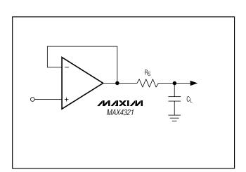
Figure 7. Capacitive-Load-Driving Circuit
