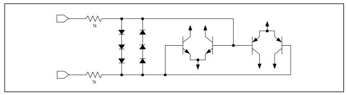
Figure 2. Input Protection Circuit
