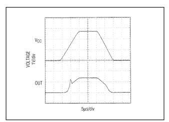
Figure 9. Power-Up Output Voltage
