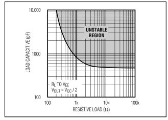
Figure 4. Capacitive-Load Stability
