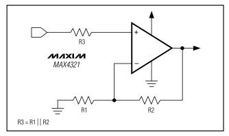
Figure 1a. Reducing Offset Error Due to Bias Current (Noninverting)
