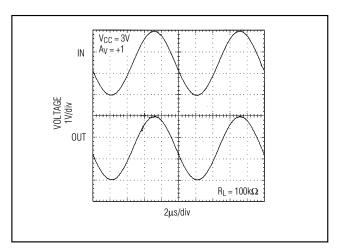
Figure 3. Rail-to-Rail Input /Output Voltage Range
