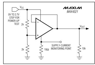
Figure 8. Power-Up Test Circuit
