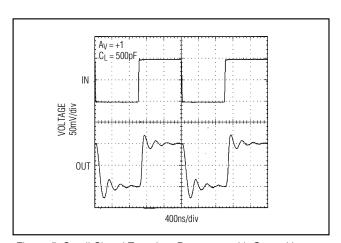
Figure 5. Small-Signal Transient Response with Capacitive Load
