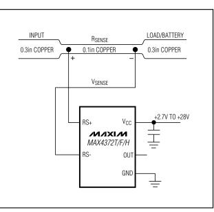
Figure 2. Connections Showing Use of PC Board
