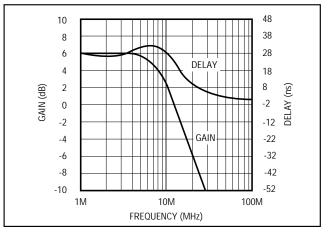
Figure 10b. Gain and Delay vs. Frequency
