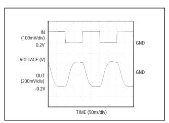
Figure 10a. 5MHz Square Wave Input
