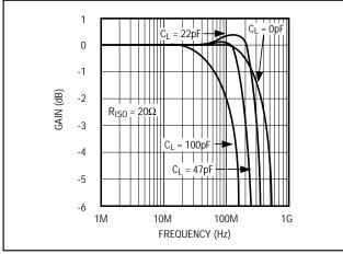
Figure 6. Effect of C<sub>LOAD</sub> on Frequency Response With Isolation Resistor
