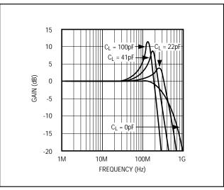
Figure 4. Effect of  $C_{LOAD}$  on Frequency Response  $(A_{VCL} = +1V/V)$
