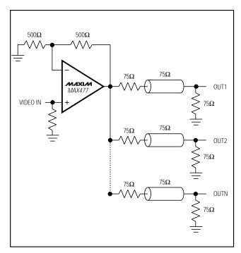
Figure 8. High-Performance Video Distribution Amplifier
