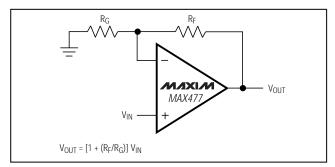
Figure 1b. Noninverting Gain Configuration
