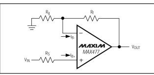
Figure 3. Output Offset Voltage
