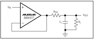
Figure 5. Capacitive-Load Driving Circuit
