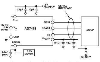
Figure 7. AD7475 Typical Connection Diagram
