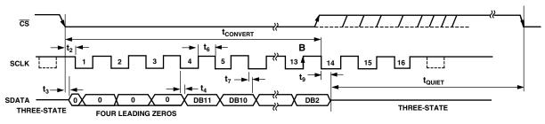
Figure 21. Serial Interface Timing Diagram-Conversion Termination
