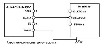
Figure 25. Interfacing to the MC68HC16
