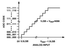
Figure 6. AD7475/AD7495 Transfer Characteristic
