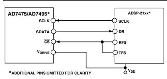
Figure 23. Interfacing to the ADSP-21xx
