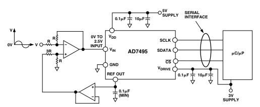
Figure 8. AD7495 Typical Connection Diagram
