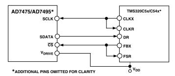
Figure 22. Interfacing to the TMS320C5x/C54x
