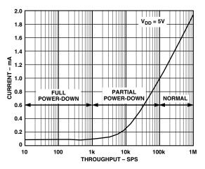
Figure 19. Typical AD7495 Current vs. Throughput
