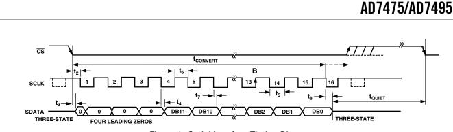
Figure 1. Serial Interface Timing Diagram
