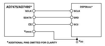
Figure 24. Interfacing to the DSP56xxx
