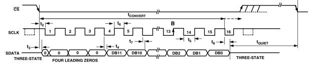
Figure 20. Serial Interface Timing Diagram
