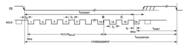
Figure 2. Serial Interface Timing Example
