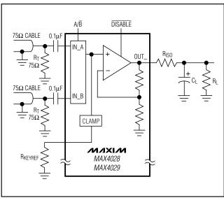
Figure 5. Using an Isolation Resistor (RISO) for a High-Capacitive Load
