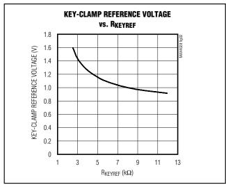
Figure 2. Key-Clamp Reference Voltage vs. RKEYREF
