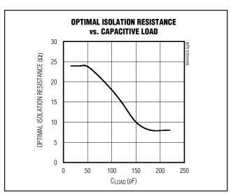
Figure 6. Optimal Isolation Resistance vs. Capacitive Load
