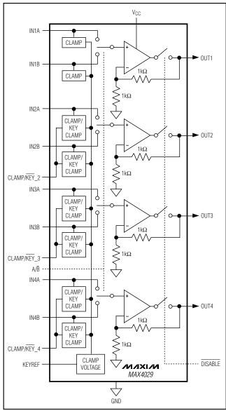
Figure 1. MAX4029 Functional Diagram
