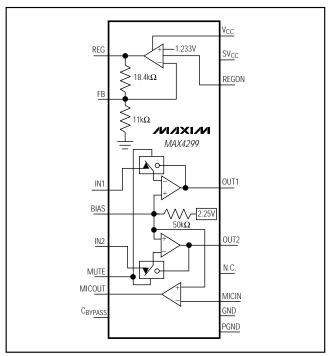
Figure 2. MAX4299 Block Diagram
