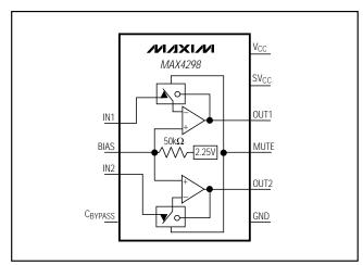
Figure 1. MAX4298 Block Diagram
