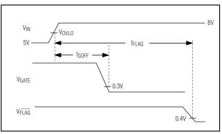
Figure 2. Shutdown Timing Diagram
