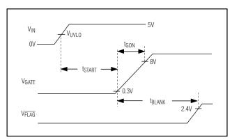
Figure 1. Startup Timing Diagram
