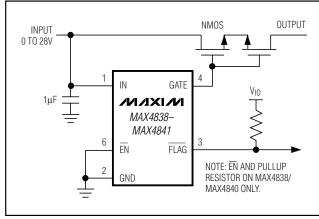
Figure 7. Back-to-Back External MOSFET Configuration
