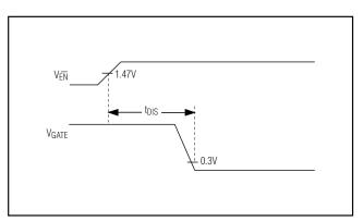
Figure 4. Disable Timing Diagram
