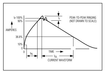
Figure 9. Human Body Model Current Waveform
