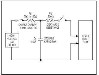
Figure 10. IEC 1000-4-2 ESD Test Model
