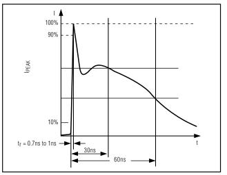
Figure 11. IEC 1000-4-2 ESD Generator Current
