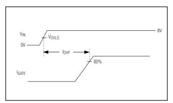
Figure 3. Power-Up Overvoltage Timing Diagram
