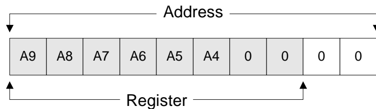
Figure 8-4. FIFO Start Address Format
