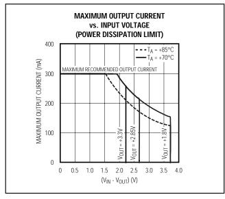
Figure 2. Power Operating Regions: Maximum Output Current vs. Input Voltage
