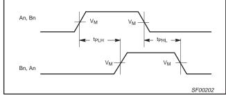
Waveform 2. For Non-Inverting Outputs
