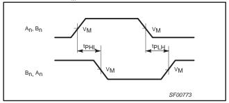
Waveform 1. For Inverting Outputs
