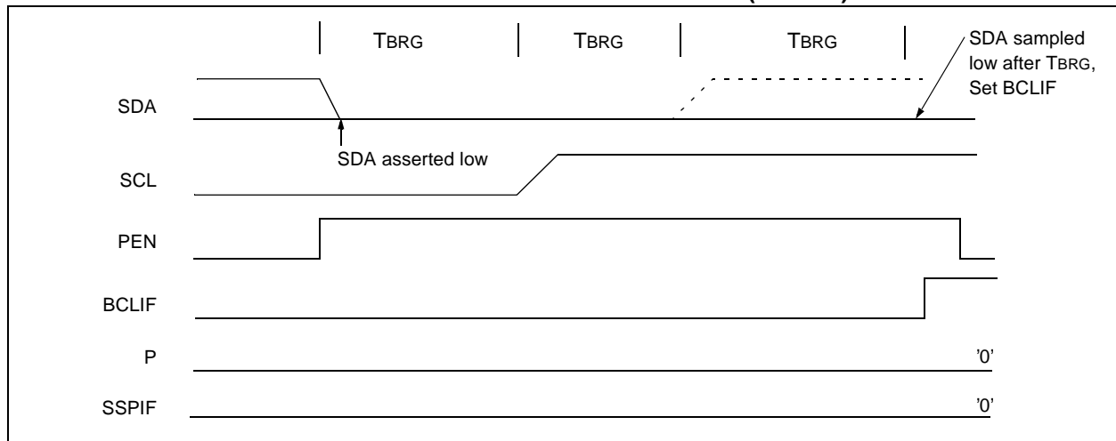
FIGURE 15-31: BUS COLLISION DURING A STOP CONDITION (CASE 1)
